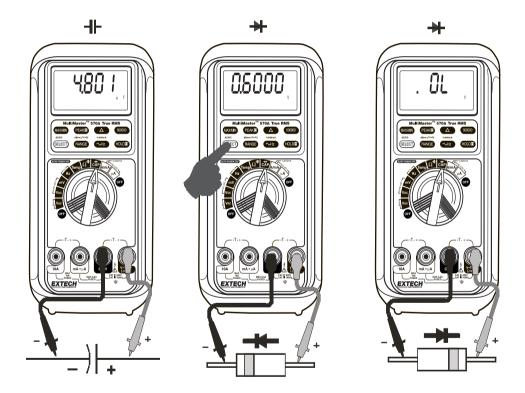
Note: Normal forward voltage drop (forward biased) for a good silicon diode is between 0.400V to 0.900V. A reading higher than that indicates a leaky diode (defective). A zero reading indicates a shorted diode (defective). An OL indicates an open diode (defective). Reverse the test leads connections (reverse biased) across the diode. The digital display shows OL if the diode is good. Any
