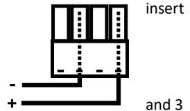
**Note:** The SD900 does not provide Loop power.
