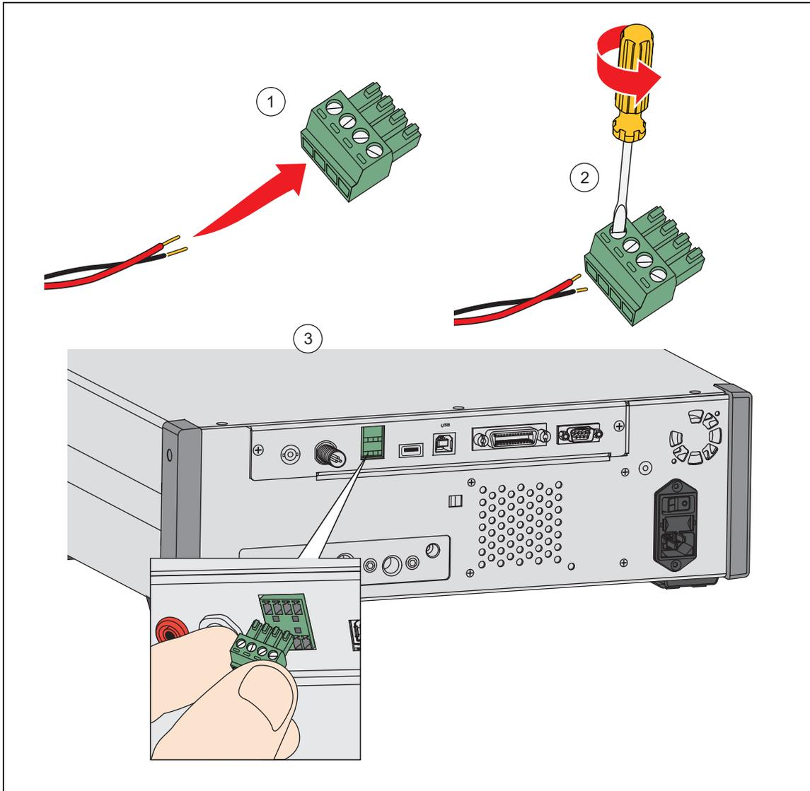
Figure 14. Driver Connections
