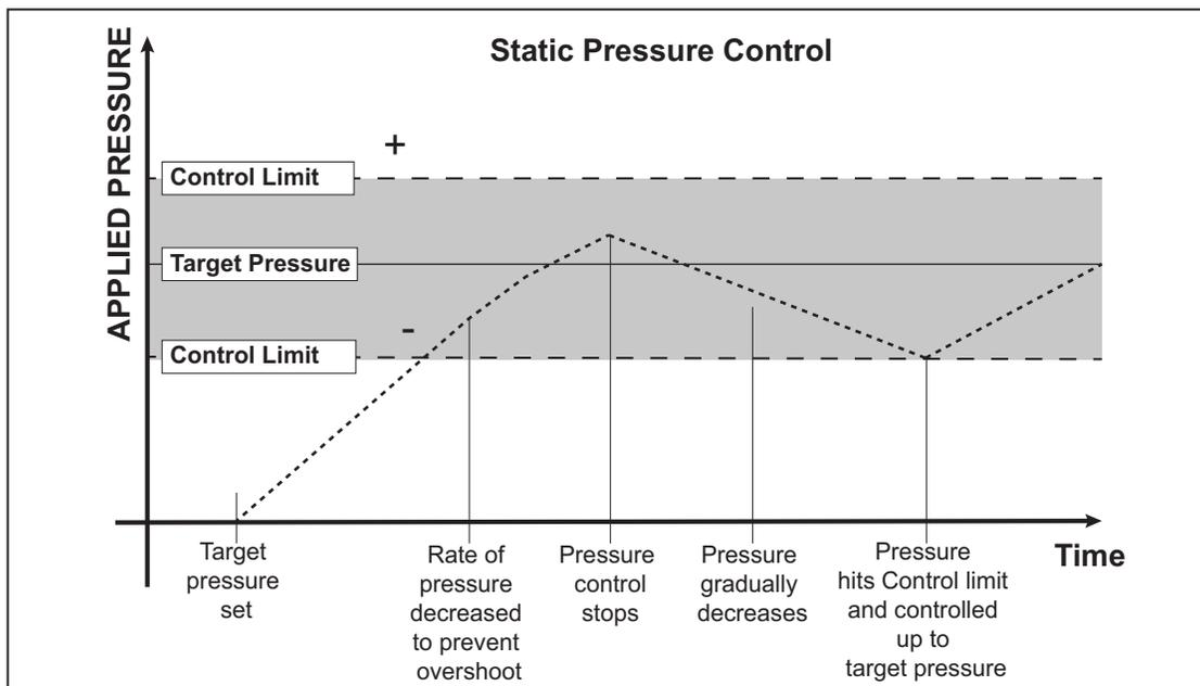
Figure 8. Static Pressure Control Mode Example
