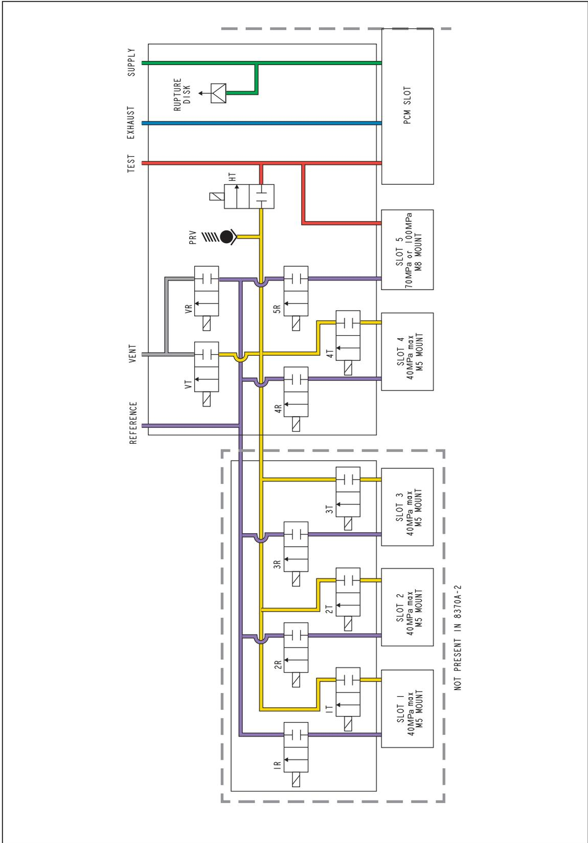
Figure 5. 8370A Pneumatic Schematic
