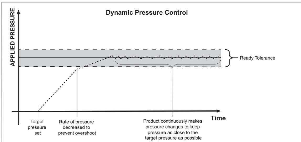
Figure 7. Dynamic Pressure Control Mode Example
