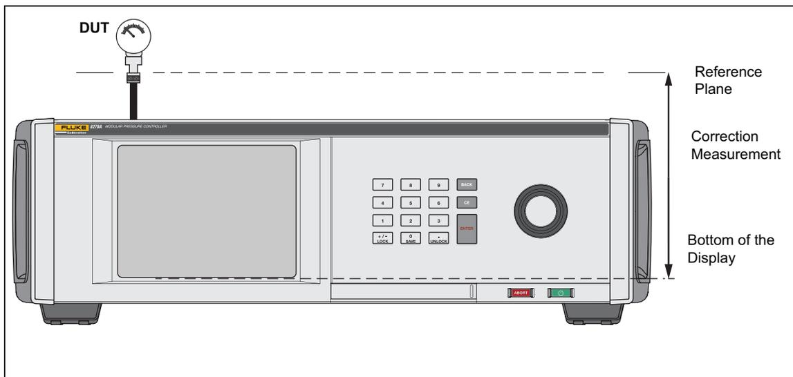
Figure 9. Head-Height Correction
