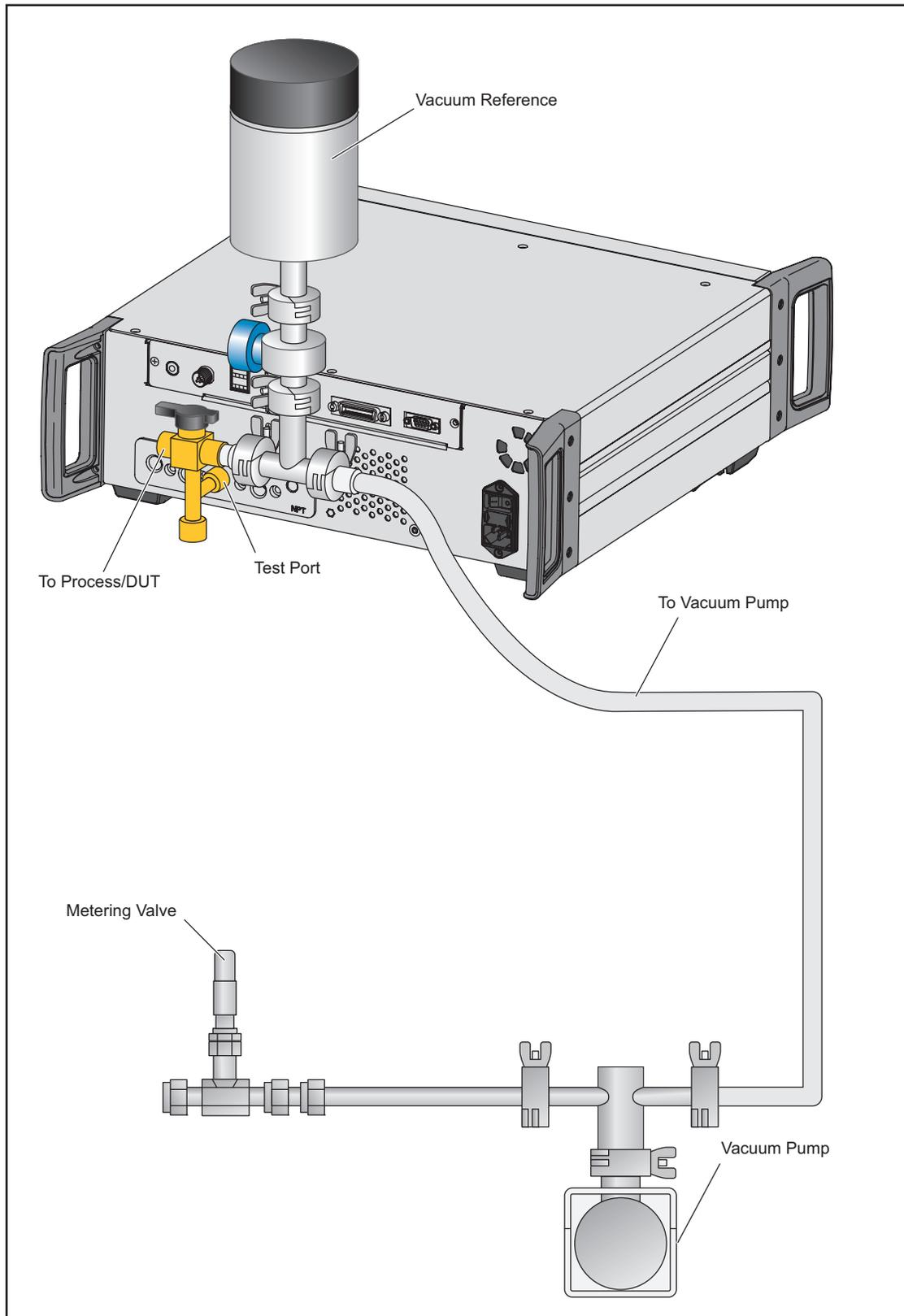
**Figure 10. Zero by Vacuum Setup**
