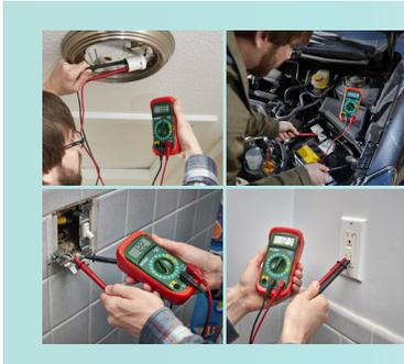
Measure AC/DC Voltage, Current, and Resistance, as well as test Diodes, Continuity, and 9 V/1.5 V batteries with this compact mini digital multimeter. The 4-digit, 2,000 count display is easy to read and the built-in tilt stand is handy for bench work. Ideal tool for the electrical hobbyist, electronics tinkerer, or DIYers working on various home improvement, vehicle wiring and A/V projects.
