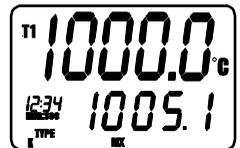
1. Press the **MX/MN** button to step through the **MX**, **MN** or **AVG** display Each reading will be accompanied by a Timer value indicating the time the reading was recorded
