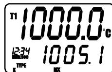
1. Press the **MX/MN** button to step through the **MX**, **MN** or **AVG** display Each reading will be accompanied by a Timer value indicating the time the reading was recorded
