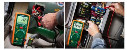
Checking voltage on a lathe and insulation test on pump motor
