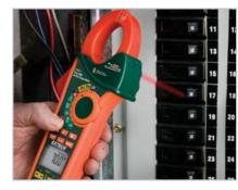
Built-in IR Thermometer for quick and safe non-contact temperature measurements.
