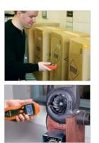
Measures the speed (RPM) of rotating objects and counts (revolution) of moving objects.
