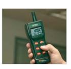
Measure CO<sub>2</sub> level in office buildings to ensure proper ventilation.
