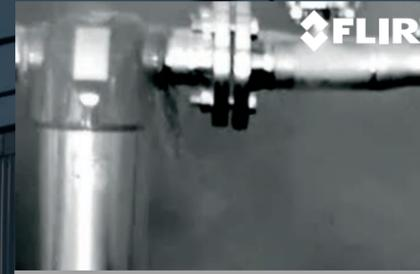
CO<sub>2</sub> LEAK - INFRARED IMAGE
