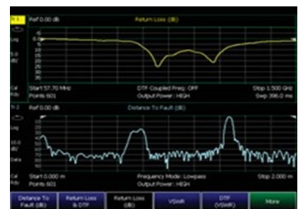
View return loss and DTF simultaneously
